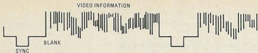
Fig. 3—COMPOSITE VIDEO SIGNAL typical of that produced by the summing network. It is a combination of raw video, sync and blanking signals generated by the IC. See text for explanation.
